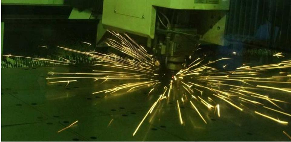
Uni-Structures' 4-kW fiber laser cuts components destined for the drive-thru.
